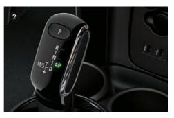
1) MINI Driving Modes. 2) Electronic gear selector lever for 7-gear double-clutch transmission.
